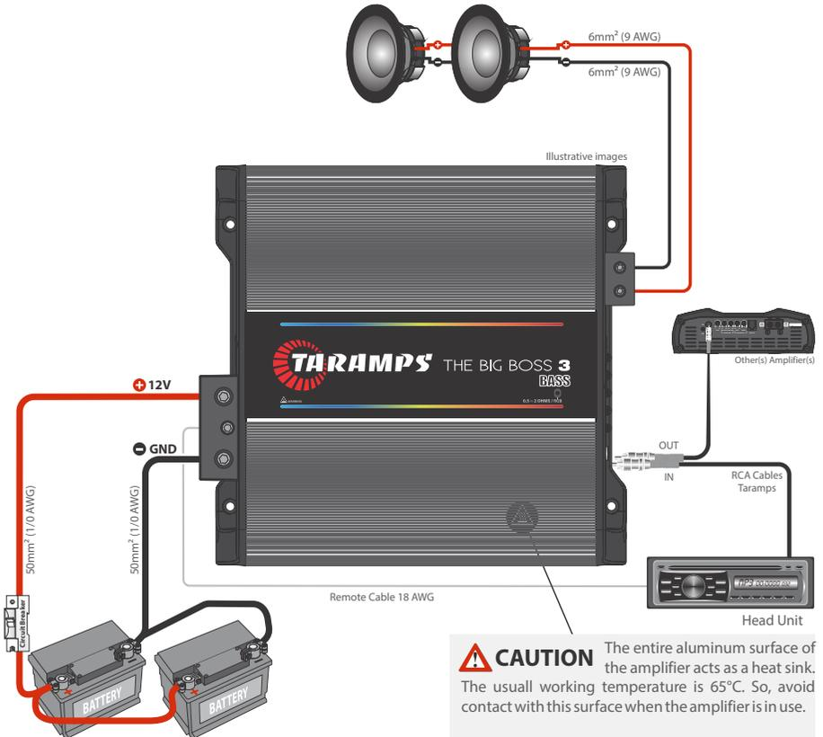
Required battery bank capacity: At least 200Ah
